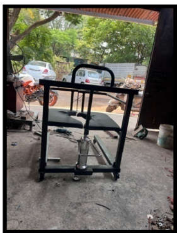
Fig 2: - Actual working model of pneumatic wheelchair
