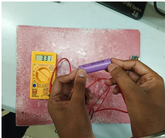
Fig. 6. Experimental setup for voltage measurement using multimeter and battery charging verification in the kinetic energy harvesting prototype
