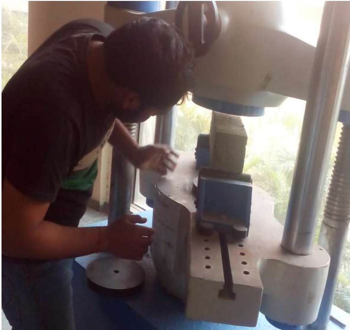
Figure 4.5: Flexural Testing of specimens using UTM
