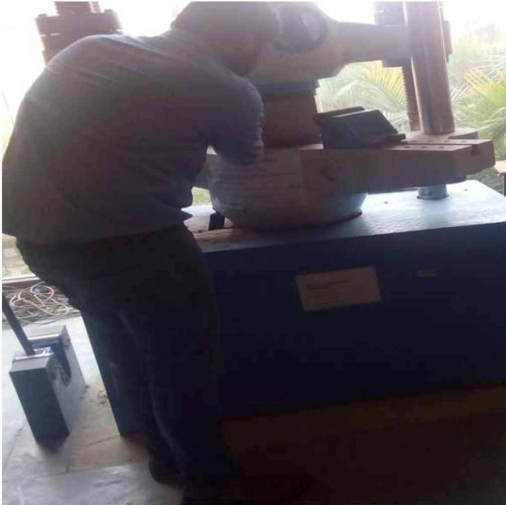
Figure 4.4: Testing of Cubes for Compressive Strength using UTM
