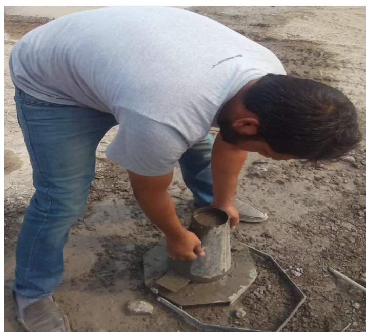
Figure 4.2: Slump Cone Testing for assessing Workability
