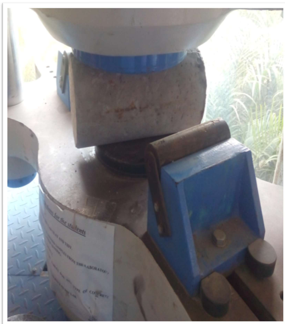
Figure 4.6: Cylinders undergoing split tensile test and curing
