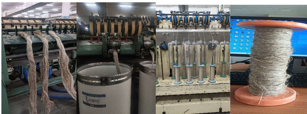
1. Drawframe(input) 2. Delivery (output) 3. Roving frame 4. Sample bobbin
